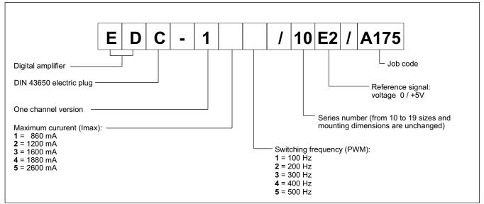
The EDC-1 connector is a digital amplifier controlling open loop proportional valves. The unit supplies a variable current in proportion to the reference signal and independently of temperature variations or load impedance.
